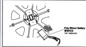
Remove the flight vehicle battery safely at the conclusion of flight .this should be made into a post flight habit to acold unforese
