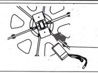
The vehicle on a flat position, the LI-PO battery in the direction shown by electrical socket pushed into position, the board flashes at this time not to move the body, so the frequency remote control gyro reading neutral point, 3 seconds after pushing the joystick to the highest, and then pulled the lowest point Receiver board lights stop flashing on the code completion
