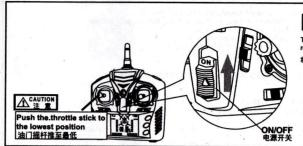
The throttle stick to the bottom, turn the remote control power
