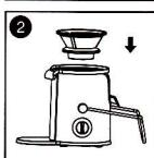
3. Place lid attached on top of receptacle, making certain it is snugly aligned with the pulp guard facing in the opposite direction of the juice spout.
