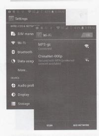
Select "Setting" and open "WLAN" function,Enter into "Wlan" and search for devices.Input the WiFi router password to connect to the device.
