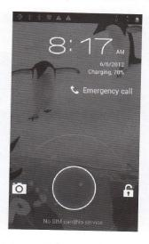
Press the power key to lock the screen.Press the POWER key/HOME key again to awaken the screen.
