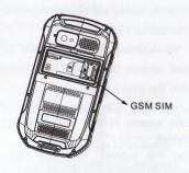
Note: When inserting the SIM card, ensure that the golden contacts faces right position.
