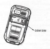
Note: When inserting the SIM card, ensure that the golden contacts faces right position.
