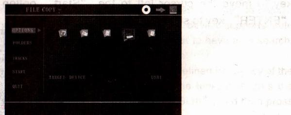
After the operation ends, press the direction key to move the cursor to the “QUIT” option and then press the “ENTER” key to exit and finally unplug the USB.
