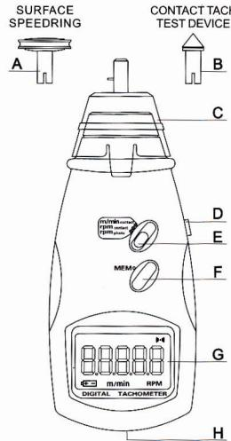
**Note:** Because of the difference between the girth of outer surface and inner flute of line speed sensor. For contact line speed or length measurement. The displaying result is correct when outer surface of the sensor contacts with the measured object contact and but when inner flute of the sensor and the measured object , that the reading multiply 0.9 is the real result (eg.: measure wire ,cable and rope etc.)
