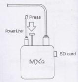
7.5 You can stop pressing the reset button until you see the android robot. And use
