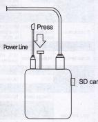
7.5 You can stop pressing the reset button until you see the android robot. And use
