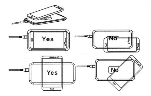
After having detected the cell phone, the charger will give out tick tuck sound and at the same time, the green device detection indicator lamp will turn on an the charge indicator lamp will keep flicking during charge.
