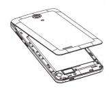
To open the back cover, lift from the bottom notch and pull up until the cover comes off.
