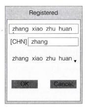
1.Number from 2-9: represent letter 2.Down key: Switch Input Method 3.Spaces key: 0 4.Up key: the delete key press up/down key to select the letters you want.
