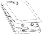
Open the notch on the lid, Then pull lightly along the lid cracks.
