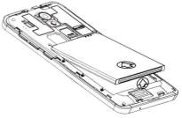
Notice: In accordance with the instructions, you should be prompted to insert,remove the batteries to avoid unnecessary damage to the body or battery.
