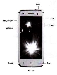
Power, To turn on/off, or screen lock/unlock Volume, Volume up/down Projector, Long press (about 3 seconds)to turn on/off projector Focus, Manual focus to make the screen clear
