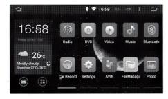
1. Go to Settings, turn on wifi function and connected to the network (open web browser, make sure the network connection is normal).
