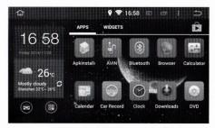
No matter which interfaces is displayed on the screen, you're allowed to click the button at the top left corner of the screen and return to the main interface. • When operating, click on the button located at top right corner of the touch screen, and then you may return to the previous screen interface.
