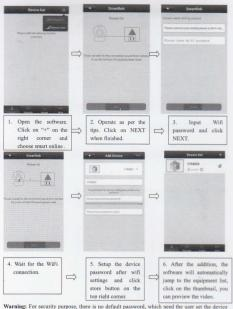
Warning: For security purpose, there is no default password, which need the user set the device password for the first time.
