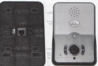
Door lock configuration instructions: PIR: Infrared Detector Call: Call Button Network: Network Status Light Power: Power Light
