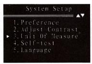
2) From *Unit of Measure* menu, use of scroll button to select the desired unit of measurement. The Unit of Measure is used in Data stream, Freeze Frame and On-Board Monitor Test.
