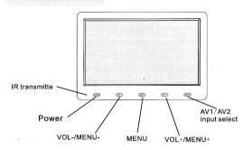
The unit use touch button, Just touch the buttons with finger to operate it.
