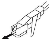
5. Release the TONEARM LOCK (3) holding the TONEARM (2) to the TONEARM REST (4) by gently pushing the TONEARM LOCK (3) to the right.
