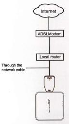
The local router LAN port with Kuluo U6 external network port via cable Connection, you can access the Internet.
