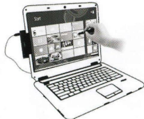
**Note:** Some notebooks have HALL-effect switch at the edge of the display, and it may cause the notebook to sleep with black screen when the magnetic metal gets close to it. Before attaching the base unit and metal strip onto the edge, please find an appropriate position to avoid interference of the HALL-effect switch.
