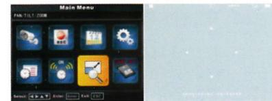
In pan/tilt/zoom menu,press enter key to enter zoom in mode,press enter again to exit zoom in mode,in zoom in mode,using <▲> key to execute up/down/left/right moving
