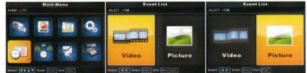
Select the entry date and hour,select the file and press enter key to play,or press Esc key and press enter key to delete the file
