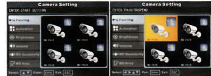
Activate  $\blacktriangle\blacksquare\blacktriangledown$  key via correspond camera icon, and press enter to perform code, and press pair key at camera side to perform code, the unit display pair ok, otherwise "no pair" after perform code, if no corresponding device pairing will esc the code pairing function press enter key within 10 seconds, can cancel the code pairing function.
