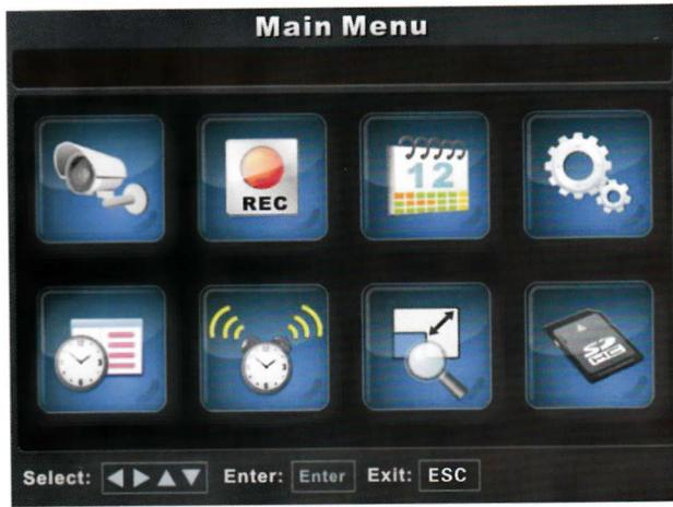
After Activate a different icon by  $\blacktriangle\blacksquare\blacktriangledown$  key press enter key to next step, press esc key to return last step.
