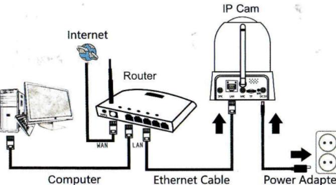
1. Connect the power adapter to the camera.
