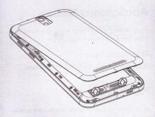
Open the notch on the lid, Then pull lightly along the lid cracks.
