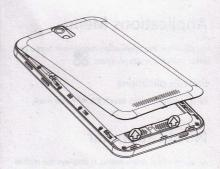
Open the notch on the lid, Then pull lightly along the lid cracks.
