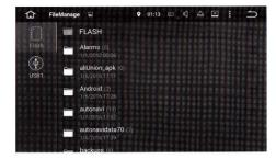
Click on the appropriate storage device (Flash, SD, GPS or USB drive) to view the files inside. Select a file or folder (file or folder after tick), then copy the key and paste the key, cut keys, between each storage device can copy, move, paste files or folders. By delete key can delete a file or folder.
