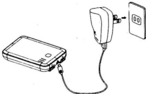
Note: While Power Station is being charged, blue LED will flash to light up. Once Power Station is fully charged, all LEDs will light up and stop charging.
