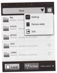
Tips: if you change the SSID and set the password, once you accidentally forgot the SSID or password, please press the power button 8 times continuous within 1.8 seconds, then the SSID and password will be restored to the default setting.
