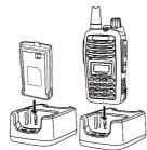
Plug the uncharged battery or transceiver with battery into charger, and make sure the battery contact with charging terminal. Red light means charging on, while green light means off.
