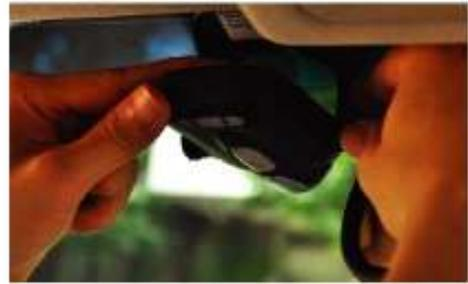
6. Connect the Power Cable to the recorder and ensure the power cable is tidy and out of the way using provided cable fitting kit.
