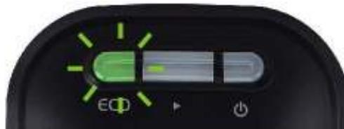
5. When the USB host back-up is completed, the Power LED will turn-off and the ECO LED will turn green.
