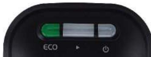
6. If there is a problem backing-up, the DVR recorder will sound and beep continuously and power LED will flicker red and the ECO LED will turn red. In this case, try again using another USB flash memory.
