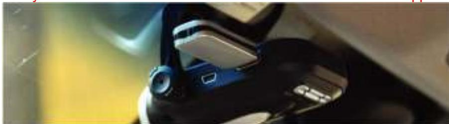
3. When a USB flash memory is connected to the DVR recorder, the POWER LED will turn-off and the ECO LED will turn blue.
