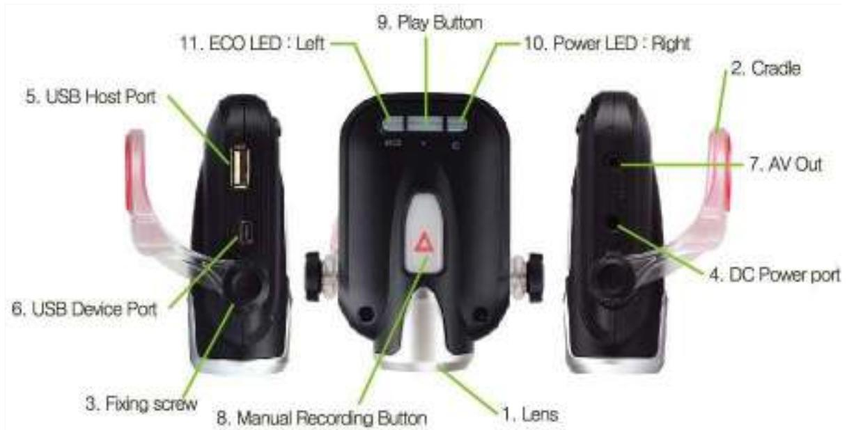
1. Camera lens: Make sure that any foreign material does not block the camera lens
