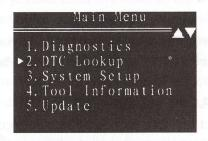
2).From *DTC Lookup* menu, hold  $\bigcirc / \bigcirc$  to move to the desired character, press  $\bigcirc / \bigcirc$  button to change selected character and press  $\bigcirc$  button to confirm. If you want to change the code to P0000, you can press  $\bigcirc$  key to clear the code.
