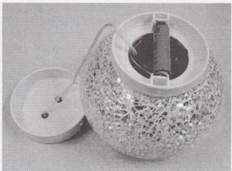
3. Remove the spent battery. Place a new "AA" size rechargeable battery into the Battery Compartment. Make sure to align the polarity indications (+/-) on the battery with those in the Battery Compartment.
