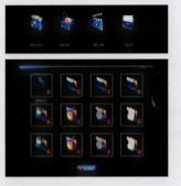
start up and enter into this screen, the press the select key, select relative mode, and the pressenter.
