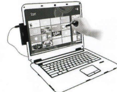
**Note:** Some notebooks have HALL-effect switch at the edge of the display, and it may cause the notebook to sleep with black screen when the magnetic metal gets close to it. Before attaching the base unit and metal strip onto the edge, please find an appropriate position to avoid interference of the HALL-effect switch.
