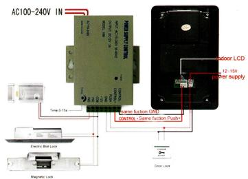
After installed, if you can't open the lock, it is possible that your wire diameter is not enough,
