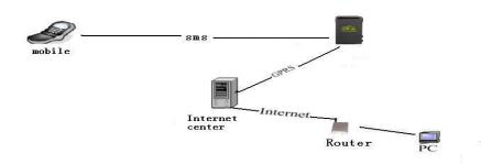
The tracker transfers GPS information to the network operator's machine room via GPRS first of all. Through wireless network, the GPS information is sent to internet and then a public IP associated with the router. The personal PC is connected with the internal network allocated by the router. In order to realize transferring GPS information to a personal PC correctly, the router must be able to transfer information received from WAN to the PCs in a LAN.
