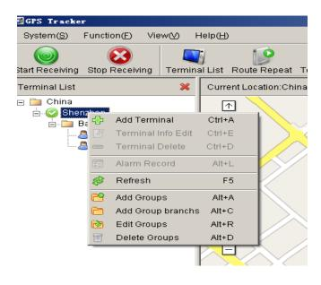
6.26. Terminal Management: Select an established terminal from the Terminal List drop-down list box and then click the right button. Users are allowed to modify the terminal/check out alarm records/add or remove terminals etc. as shown below:
