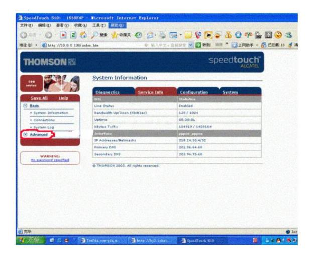
6.7.5.2 When logging in, the basic interface of ALCATEL511 appears and then click the column ADVANCED in the left of the screen
